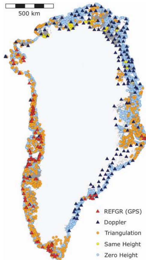
Figure 2. Ground control used in the aero-triangulation of the photographs. Triangulation points indicate ground control with coordinates and heights assigned by GPS or Doppler-based adjustment of the terrestrial triangulation network. Ground control outside of these networks is not connected to triangulation networks.
