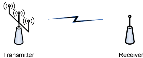
Figure 2.4 A multiple input - single output system.
