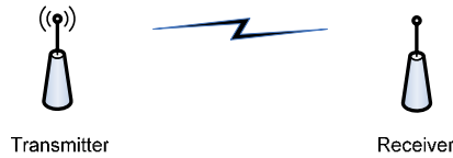
Figure 2.1 A conventional SISO communications system.
