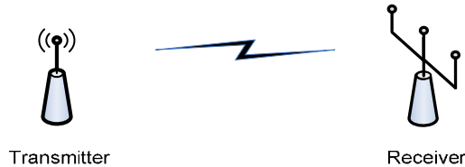
Figure 2.3 A single input - multiple output system.
