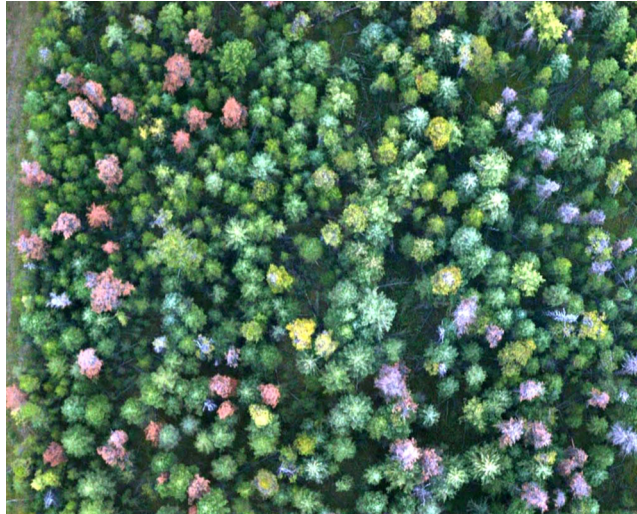
Fig. 1 A sample of VHSR airborne imagery showing various stages of mountain pine beetle infestation (as manifested in the color of the crown). Once a tree is killed by mountain pine beetle, the foliage will gradually fade from green (green-attack stage) to greenish-yellow (faders) to red (red-attack stage) over the spring and summer following attack. The needles will slowly drop until the tree is completely defoliated (gray-attack stage).
