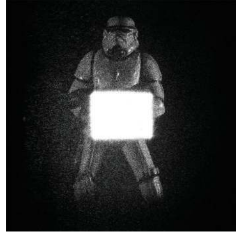
FIGURE 2: Reconstructed DH of a Starwars schart. Note the presence of the both the DC terms and the conjugate image term.
