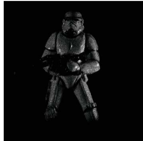
FIGURE 7: This reconstruction is the same as Figure 5, where both the conjugate image term and the DC terms have been removed. Unlike in the numerical procedure used in Figure 5, we have applied a PSI technique to separate out the real image term.
