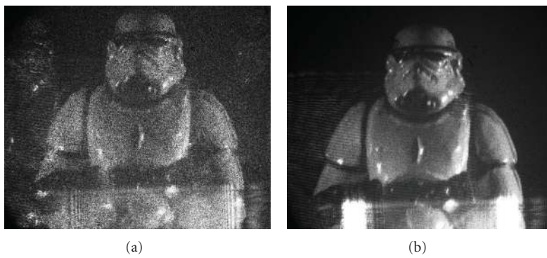
FIGURE 16: Removal of speckle noise in optoelectronic reconstruction by CCD integration of reconstructed images: (a) reconstruction from one image, (b) reconstruction from ten images.
