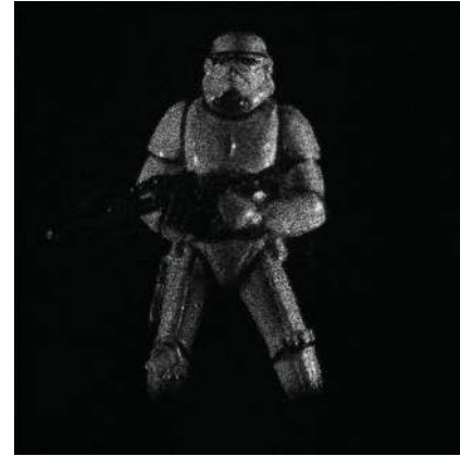
FIGURE 5: This reconstruction is the same as Figure 2, however both the conjugate image term and the DC terms have been removed using numerical processes described in the text.
