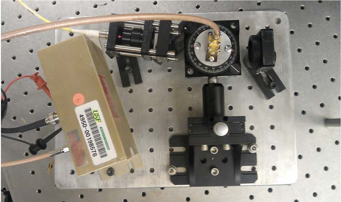
Figure A.3. Acousto-Optic Modulator (AOM) shutter system. Imaging beam enters from HeNe source through fiber optic from left, is condensed through AOM and diffracted (when triggered by driver) through iris and collimating lens exiting to the right.
