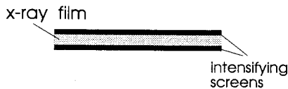
Fig. 1 Principle of conventional x-ray image detection by a screen/film combination. The light-sensitive film is sandwiched between two phosphor intensifying screens which convert the incoming x radiation into visible light.
