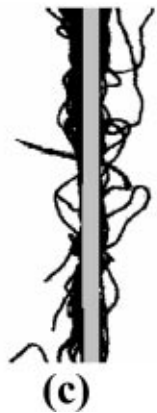
Fig. 15 (a) Dark-field yarn image, (b) integration of a 1 mm section for each column on a dark-field image showing the selection of core edges, (c) and (a) after hair-core background separation.
