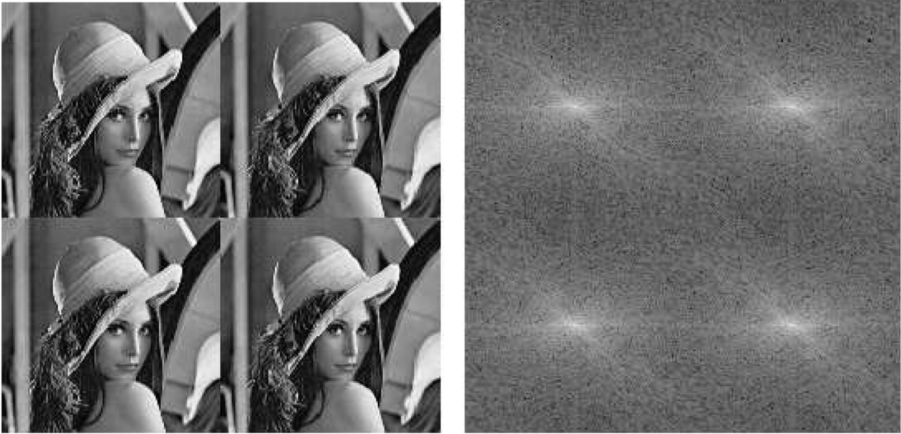
Fig. 8. Balanced multiwavelet approximation subband of Lena image (left). Spectral densities of subband blocks L_0L_0 , L_0L_1 , L_1L_0 , and L_1L_1 (right).
