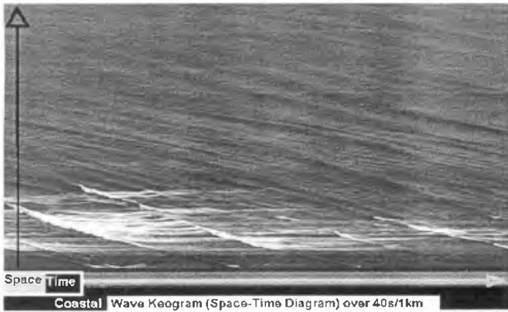
Figure 3a illustrates the horizon fix, GPS landmark selection and video sampling line placement. The keograms which follow illustrate the time stack output of the intensity profiles extracted from the sampling line at the full TV frame rate and averaged in order to focus on the phenomena of interest. (For details see the appendix at the end of the chapter.
