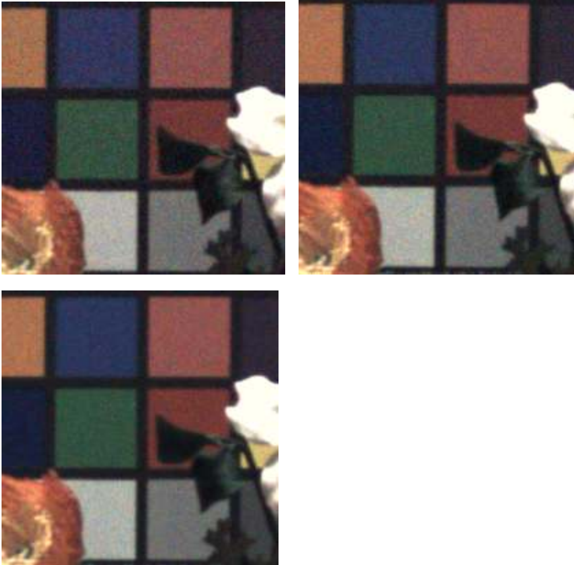
Figure 3.18: Detail of SNR=30 image section after correction by methods: Top Left: Optimal 3x3 Matrix, Overall SNR=35, 18% Gray SNR=15, Top Right: ST, Overall SNR=37, 18% Gray SNR=16, Bottom: SCLS SNR, Overall SNR=42, 18% Gray SNR=18.
