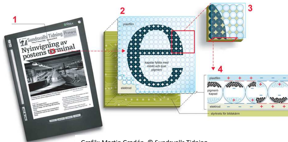
Figure 1. The principle of e-paper displays
