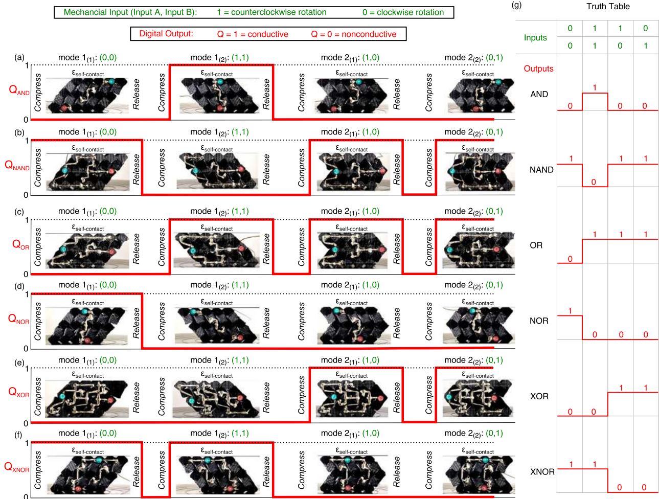
Fig. 5 Processing all digital logic operations in soft, conductive mechanical metamaterials. Logic gate digital output Boolean response at each of the four compact states for the (a) AND, (b) NAND, (c) OR, (d) NOR, (e) XOR, and (f) XNOR logic gate. The respective mechanical inputs (green) for each of the deformation states directly relate to (g) the logic gates truth table inputs.
