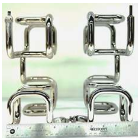
FIGURE 6. Polymerized bound sand with plating.
