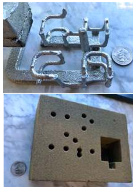
FIGURE 7. Cast aluminum with a 3D printed sand mold.
