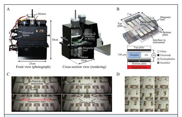
Fig. 1. Automated digital microfluidic platform.
