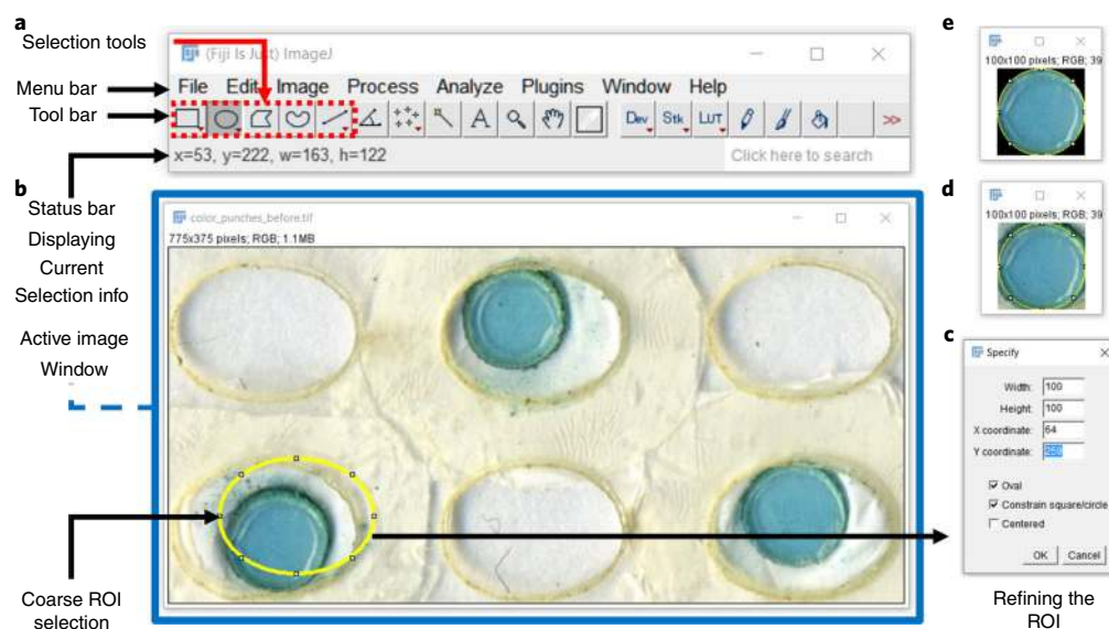
Fig. 4 | Overview of the ImageJ GUI and ovoid ROI selection, refinement and cropping. This figure features an image of 2.5-mm laser cutouts of plastic-backed, silica thin-layer chromatography (TLC) plates. The circular, TLC plate cuttings were treated with malachite green and placed in individual microfluidic chambers for colorimetric, organophosphate detection and differentiation. Subgroups of organophosphates, namely chemical warfare agents and pesticides, are highly deleterious to human health either through terroristic use or accidental consumption. Shown here, we demonstrate how to select, refine and crop an ROI using the ImageJ GUI. a , The ImageJ GUI consists entirely of the menu, tool and status bars. Selection tool icons are accessible directly from the tool bar (red box). b , Dragging-and-dropping an image file directly onto the status bar opens a new window containing the active image. Similarly, images can be opened via the File > Open... submenu. Clicking the oval selection tool icon allows the user to define a circular/ovoid ROI by clicking-and-dragging on the active image (yellow outline). Clicking-and-dragging the handles on the selection permits coarse refinement of the ROI. c , The Edit > Selection > Specify submenu permits further refinement and modification of the current ROI selection. d , After refining the ROI selection, the active image is cropped via keyboard shortcuts (Ctrl + Shift + X) or the Image > Crop submenu. Notice that ImageJ crops the image to a rectangle that completely bounds the active selection. e , The area outside the ROI selection is removed via the Edit > Clear Outside submenu.
