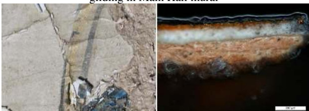
Figure 11 the microscopic cross-sectional structure of the gilding in Guan Yin Hall mural
