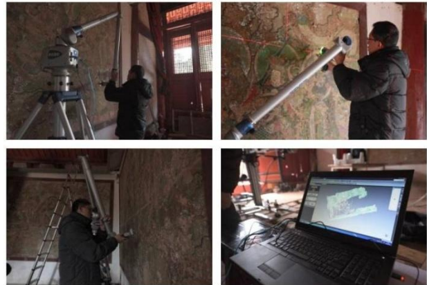
Figure 22 use arm of a laser scanner to develop a good 3D model of the mural surface
