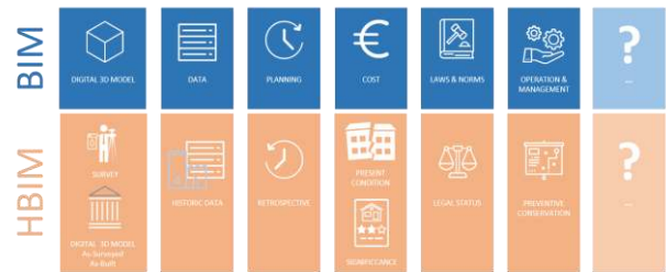
Figure 1 – The figure depicts the type of information that should be integrated in HBIM data model in comparison with standard BIM data models.
