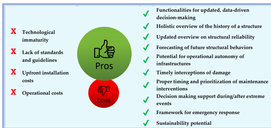
Figure 4. Pros and cons of a Digital Twin implementation in a civil engineering system from an infrastructure manager perspective.
