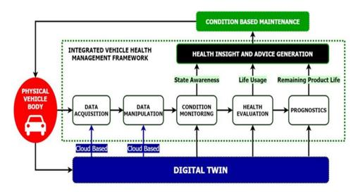
Figure 5. Digital Twin technology embedded within the MRO.
