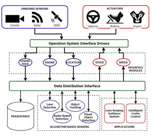
Figure 4. Driver's assistance system architecture.
