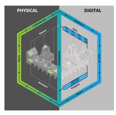
such system layouts have apparently become virtual rather than physical. Figure 2 depicts a characteristic systemic layout of a digital twin [10,11].
