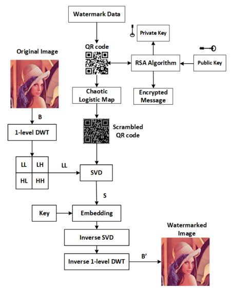
Figure 4. The proposed scheme: embedding process.
