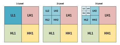
Figure 2. Three levels of DWT decompositions.
