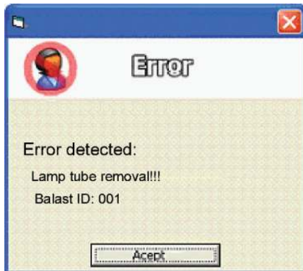
Figure 11. Fault condition window for lamp tube removal
