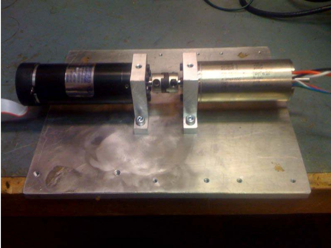
Figure 5-6 – Mechanical Test Rig with DC motor drive on the left and 3-phase generator shown on the right
