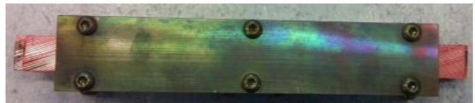
Fig. 3: Bare cable stack in its reaction fixture.
