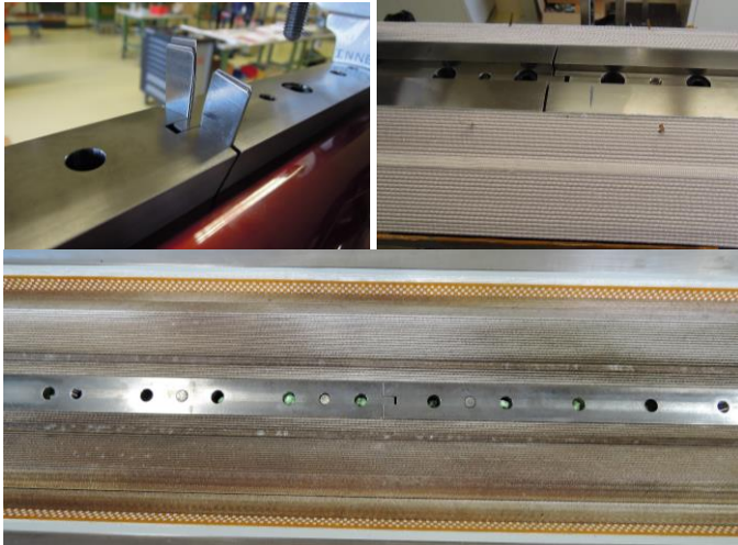
Fig. 6: Gaps in the pole at different steps. Top left: gaps set with controlled shims. Top right: gap remaining after release of the winding tension. Bottom: gaps almost closed after reaction.
