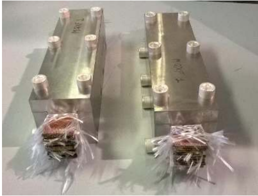
Fig. 4: Insulated cable stacks in the reaction fixture, before heat treatment.
