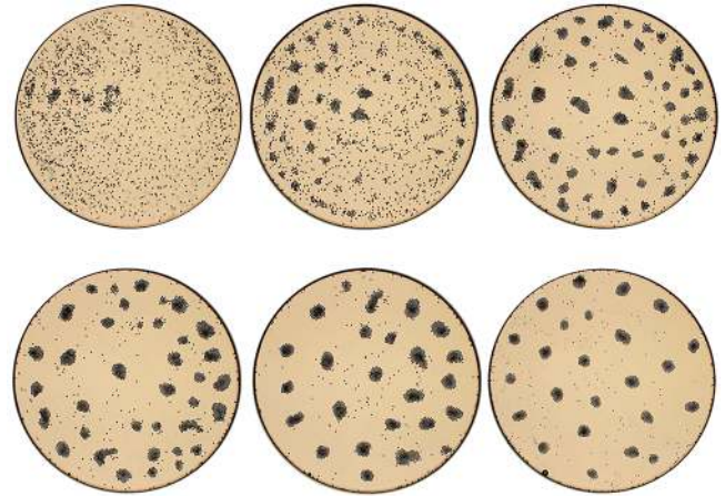
Fig. 4. Time lapse of one experiment over the course of 30 min. The height of the reservoir is 2 mm, the reservoir diameter is 6 mm, the initial particle diameter is 45 \mu\text{m} , and the surfactant concentration c_s is 10 wt%. Top row from left to right: 0, 1 and 3 min. Bottom row from left to right: 5, 10 and 30 min.
