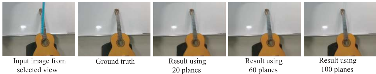
Fig. 14 Comparison of using the different number of planes to render output images.
