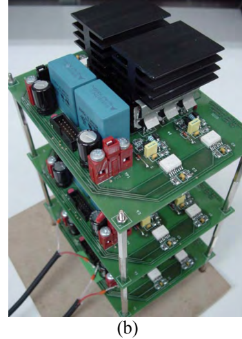
Fig. 5: Three-level three-leg dc-ac converter. (a) Topology. (b) Prototype using 150 V MOSFETs as devices S_{xi} .
