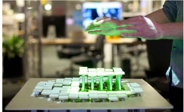
Figure 1: We propose to extend direct touch interaction with 2.5D shape displays by a set of free-hand gestures
