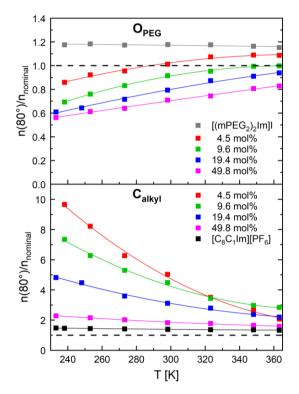
**Figure 4.** Normalized content  $n(80^\circ)/n_{nominal}$  for  $O_{PEG}$  (**top**) and  $C_{alkyl}$  (**bottom**), derived from the corresponding  $80^\circ$  intensities and their nominal atomic numbers of  $O_{PEG}$  and  $C_{alkyl}$  for the pure ILs and mixtures for different temperatures (measurements started at 363 K).
