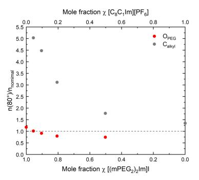
**Figure 3.** Normalized content  $n(80^{\circ})/n_{nominal}$  for  $O_{PEG}$  (red) and  $C_{alkyl}$  (grey), derived from the corresponding  $80^{\circ}$  intensities and the nominal atomic numbers of  $O_{PEG}$  and  $C_{alkyl}$  for the pure ILs and mixtures at T = 298 K.
