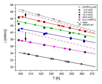
**Figure 5.** Surface tension values measured using the PD method are shown as open and full squares, along with their linear fits (lines) using Equation (1). The surface tension values calculated from the 80° ARXPS data using Equation (3) are shown as filled circles. Furthermore, the ideal behaviour for the surface tension of the 4.5 and 49.8 mol% mixtures as determined by Equation (2) (dashed lines) is included for comparison (a comparison for all mixtures is shown in Figure S4).
