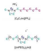
**Figure 1.** Structure of 1-methyl-3-octyl-imidazolium hexafluorophosphate  $[C_8C_1Im][PF_6]$  (**top**) and 1,3-bis(polyethylene glycol)imidazolium iodide  $[(mPEG_2)_2Im]I$  (**bottom**). The different carbon atoms giving rise to the three discernible C 1s peaks are color-coded in blue (C<sub>2</sub> peak), in turquoise (C<sub>hetero</sub>), and in pink (C<sub>alkvl</sub>).
