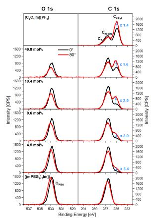
**Figure 2.** O 1s and C 1s spectra at  $0^{\circ}$  (black) and  $80^{\circ}$  (red) emission of pure [C<sub>8</sub>C<sub>1</sub>Im][PF<sub>6</sub>], pure [(mPEG<sub>2</sub>)<sub>2</sub>Im]I, and of different mixtures of these ILs, collected at T = 298 K. The relative increase in C<sub>alkyl</sub> intensity upon changing the emission angle from  $0^{\circ}$  to  $80^{\circ}$  is indicated (for details, see text).
