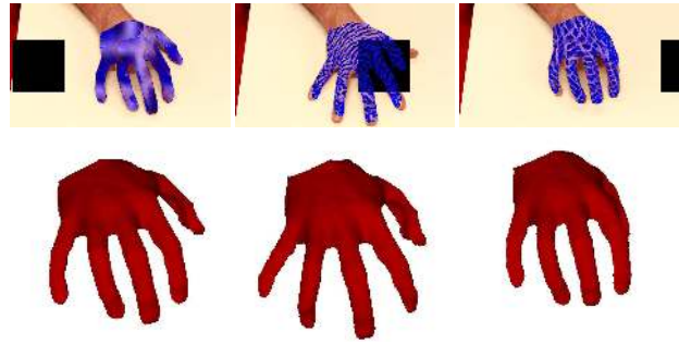
Figure 10: Occlusion experiment on hand sequence. Here it can be seen that the hand motion is reliably estimated despite the presence of a large occluder.
