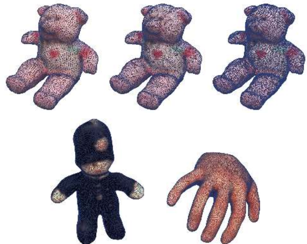
Figure 5: An example of our multi-scale template meshes generated by iterative mesh down-sampling and refinement. Top: From left to right the meshes contain approximately 5, 10, and 25 thousand vertices respectively. Bottom: The highest levels of the templates for the bobby and hand sequences.
