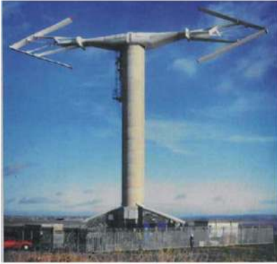
Figure 2.4: To the left is an H-rotor developed in the U.K. and to the right is one of the Heidelberg rotors.
