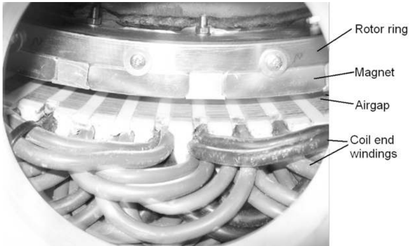
Figure 4.6: Close view of the generator taken on the first experimental generator.
