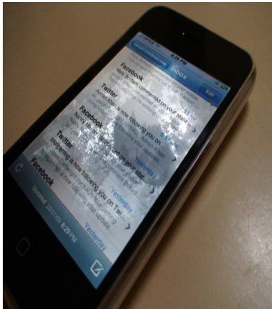
Figure 12: Water damage behind cover glass of iPod.
