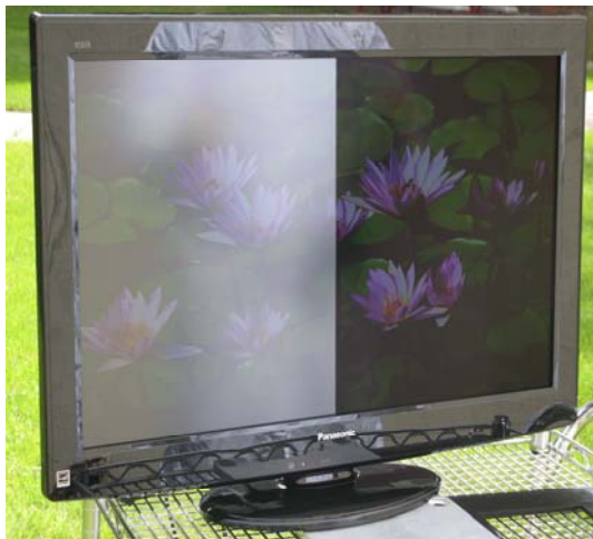
Figure 5: Example of standard 32" TV with half air gapped (left) and half bonded (right) with HEA cover glass. The Specular reflectance was reduced from 1.46% to .42%.
