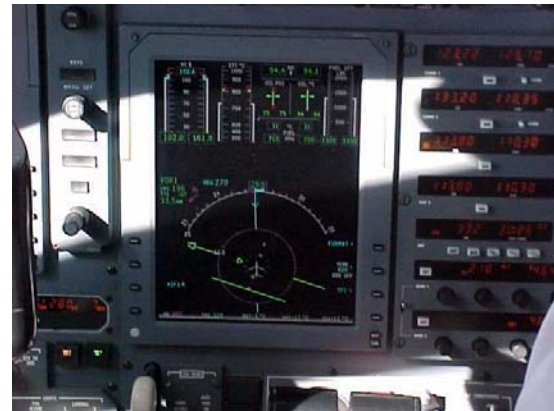
Figure 6: Example of Shafted Sunlight in a cockpit with Laminated Display
