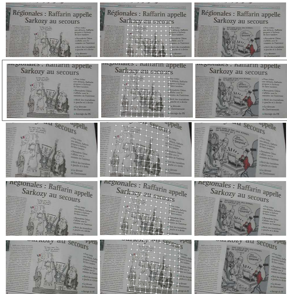
Figure 5: Registration results on the Newspaper sequence. (left) Original images. (middle) A mesh grid illustrating the computed mapping. (right) The cartoon on the reference image (indicated by a black frame) is replaced and mapped onto the other frames.
