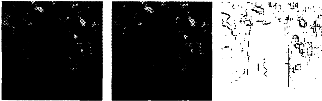
Figure 23: a) The result of filling in the updated depth map with threshold \min + \sigma , b) MRF smoothing of filled in depth map, c) line processes
