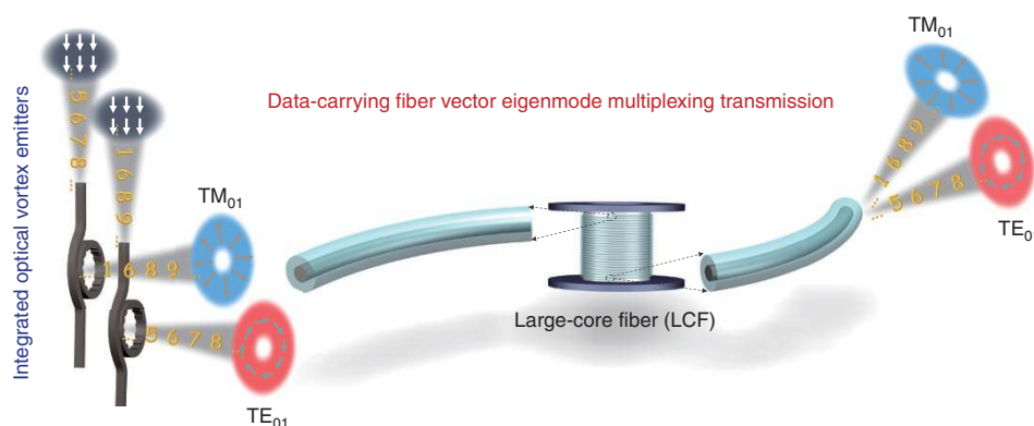
Figure 1 Conceptual illustration of data-carrying fiber vector eigenmode multiplexing transmission seeded by integrated optical vortex emitters. Two data-carrying fiber vector eigenmodes with polarization vortices, that is, radially polarized mode ( TM_{01} ) and azimuthally polarized mode ( TE_{01} ) generated using silicon microring resonators with the inner sidewall etched as angular gratings, are multiplexed and transmitted through a large-core fiber (LCF) for increased transmission capacity and separated after transmission with low-level crosstalk.
