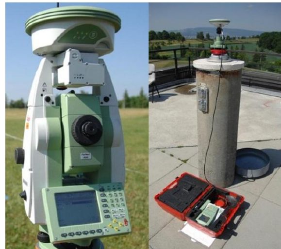
Figure 2. GPS reference station with Leica GPS1200 (right) and Leica SmartStation (left) during data acquisition.
