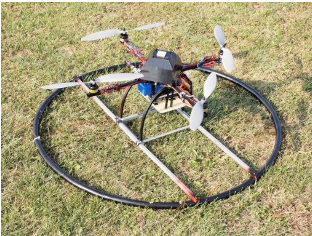
Figure 1: UAV system based on the 'MikroKopter' project.
