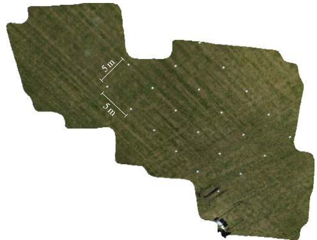
Figure 6: Test area with 24 control points on a model aircraft field.
