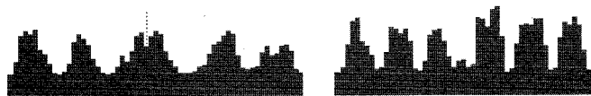
Fig. 6. The figure shows two sections, belonging to regions with different ridge line density. The dotted line denotes the point where a ridge center (hence, a local maximum) should exist. On the contrary, the image noise originates, in that point, a local minimum which produces a typical volcano silhouette.
