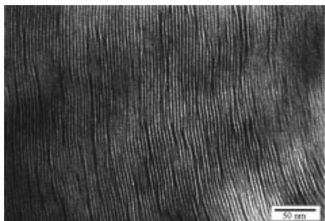
Figure 4. TEM micrograph of P4VP-NPD 1.0 illustrating the lamellar structure with a long period of ca. 40 Å.
