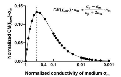
**Figure 7.** Normalized Clausius–Mossotti (CM) factor multiplied by conductivity of the medium versus normalized conductivity of medium in the low frequency range below 100 MHz. The conductive behavior dominates the value of the CM factor and the DEP force is attractive (see [44], their Section 2.4.1).
