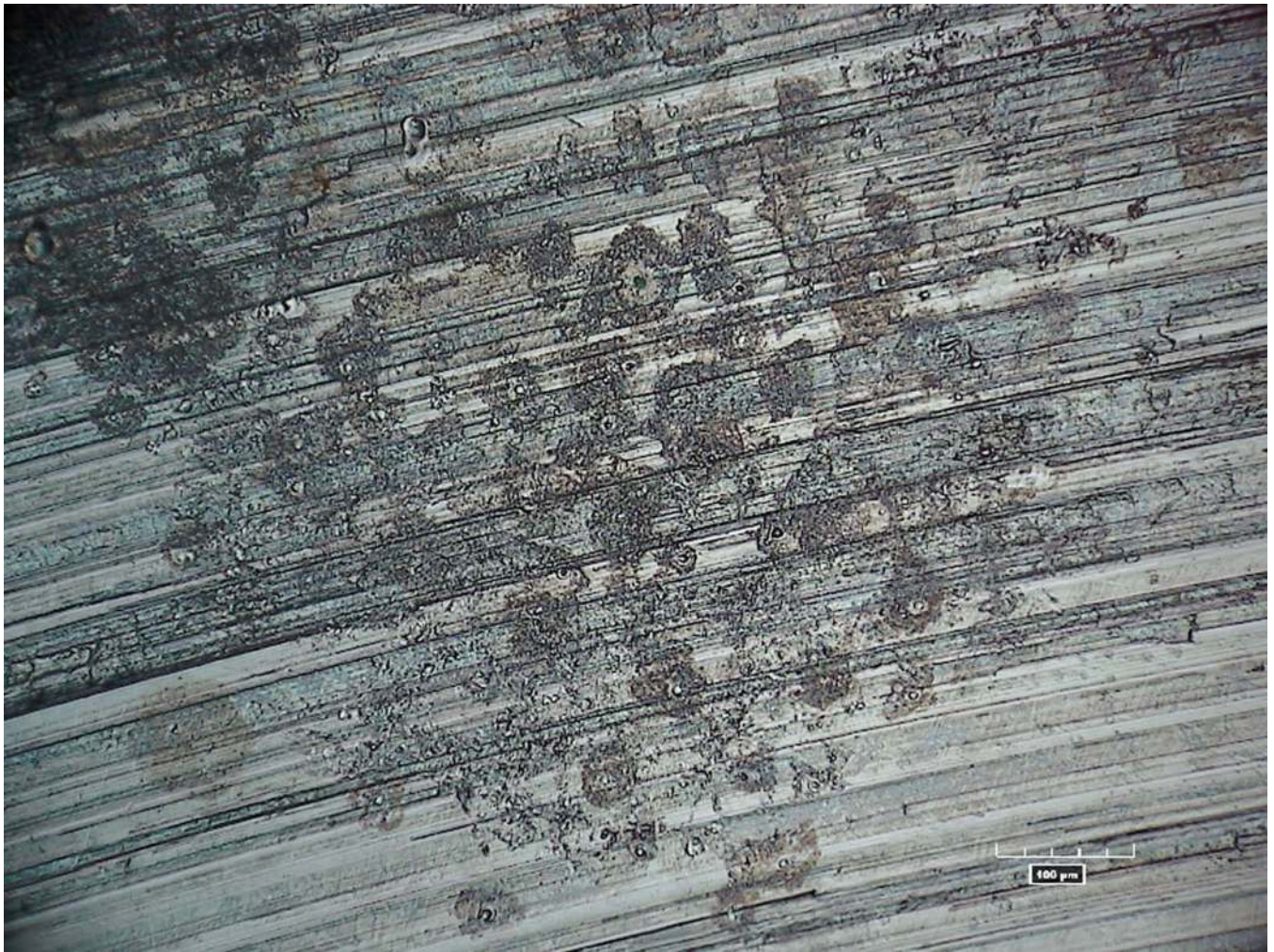
Figure 6. Digital optical micrograph of a CoCrMo head where ICI corrosion has taken place on a non-articulating machined surface adjacent to the modular taper bore. Machining lines are damaged by the ICI corrosion process in patterns consistent with the ICI corrosion seen in earlier examples on articular surfaces. The modular taper bore is about 3 mm to the lower right.
