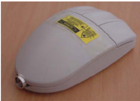
Figure 8: An infrared laser pointer enclosed in a mouse case.
