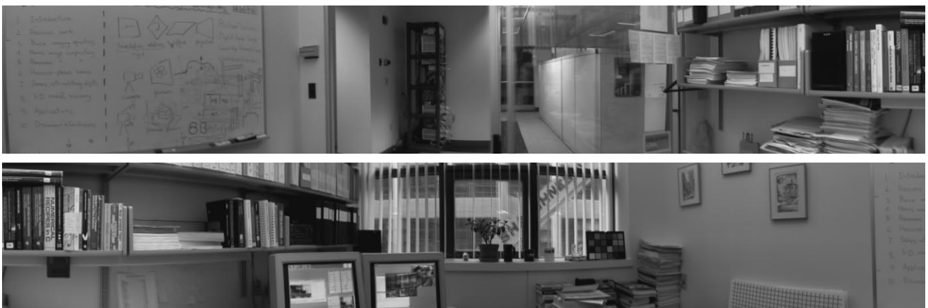
Figure 3: Circular panoramic image mosaic example (office interior). A total of 36 images were pasted onto a cylindrical viewing surface.
