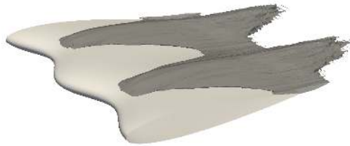
Figure 13: Iso-surface of TKE = 0.015 for wavy wing with \alpha = 6^\circ and Re = 50\,000 .
