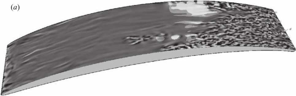
FIGURE 40. Simulation T3: contours of the wall-normal velocity perturbations -0.01 < u'_n < 0.01 at a distance d \sim 1.64 \times 10^{-3} from the suction surface. The highlighted perturbation amplifies and leads to breakdown, in a manner similar to the instability in figure 35 for simulation T2.
