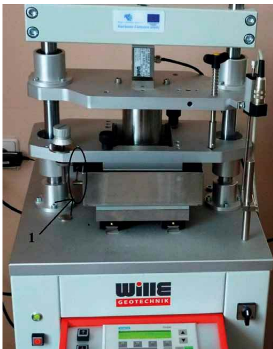
Fig. 3. Direct shear apparatus. 1 – external horizontal displacement transducer
