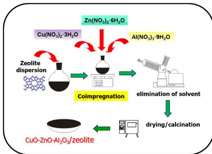
Figure 13. Scheme of the preparation of Cu-ZnO-Al 2 O 3 /zeolite catalysts for direct synthesis of DME using co-precipitation method.
