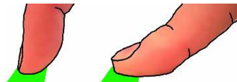
Figure 11. The changing contact area results in a non-uniform mapping between fingertip and point of interaction.
