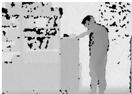
Figure 1. Example of imperfections in a Kinect depth map: Original depth map with hole pixels (represented as black pixels) detected by the “non-available” tags.
