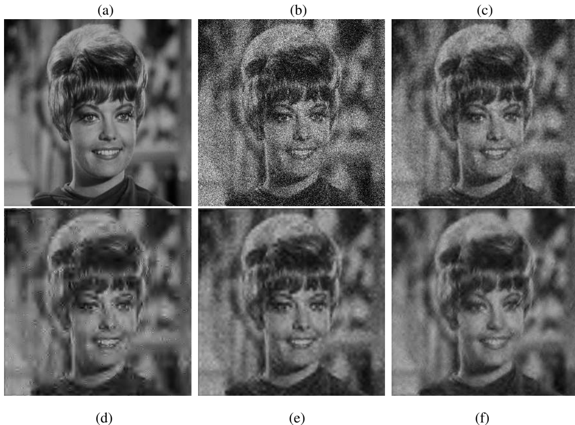
Fig. 13. Denoising results of “Zelda” image: (a) “Zelda” image, (b) noisy image (noise standard deviation = 50, PSNR = 14.61dB), (c) wiener2 (PSNR = 25.78dB), (d) wavelet thresholding (PSNR = 26.05dB), (e) wavelet HMT (PSNR = 27.63dB), and (f) contourlet HMT (PSNR = 27.07dB).
