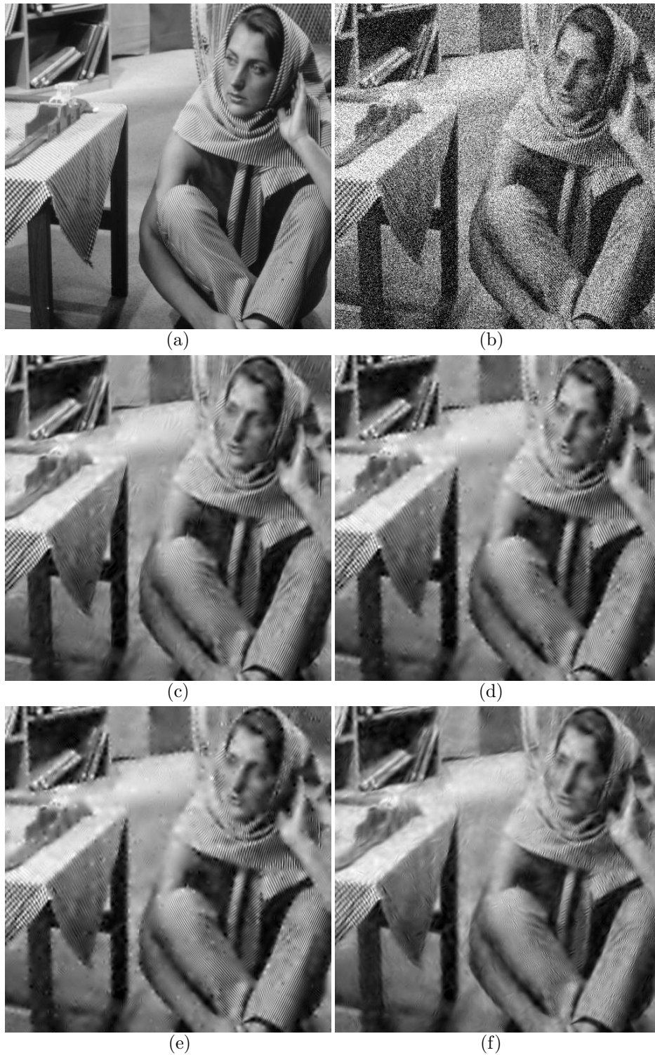
FIGURE 14. Denoising experiments with a Barbara image. (a) Original image. (b) Noisy image with \sigma = 50 , PSNR=14.20 dB. (c) Restored image using ab-shear, PSNR=25.59 dB. (d) Restored image using c-hyper, PSNR=25.78 dB. (e) Restored image using hyper, PSNR=25.35 dB. (f) Restored image using ab-star, PSNR=24.06 dB.
