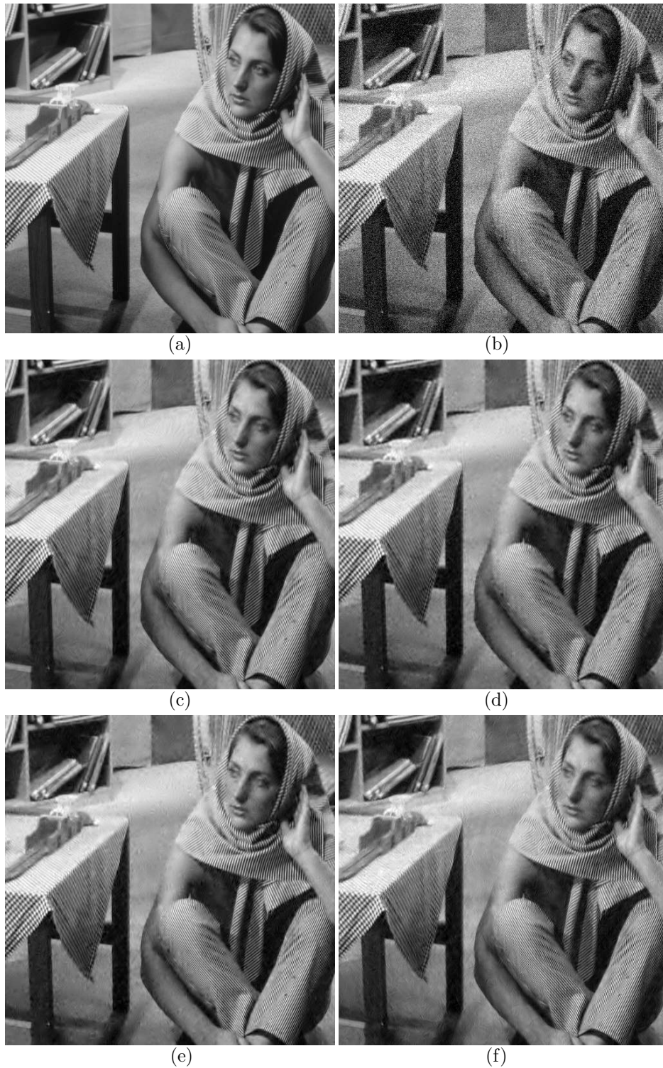
FIGURE 13. Denoising experiments with a Barbara image. (a) Original image. (b) Noisy image with \sigma = 20 , PSNR=22.15 dB. (c) Restored image using ab-shear, PSNR=30.38 dB. (d) Restored image using c-hyper, PSNR=30.41 dB. (e) Restored image using hyper, PSNR=30.49 dB. (f) Restored image using ab-star, PSNR=29.02 dB.
